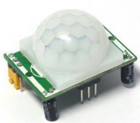
Figura 2-4: Sensor PIR HC-SR501
