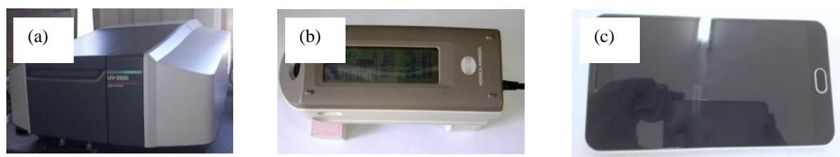
Figure 3. 20 (a) Spectrophotometer used for reflectance UV-vis measurements, (b) portable spectrophotometer used for CIELab color measurements, and (c) Mobile phone used for make digital images.
