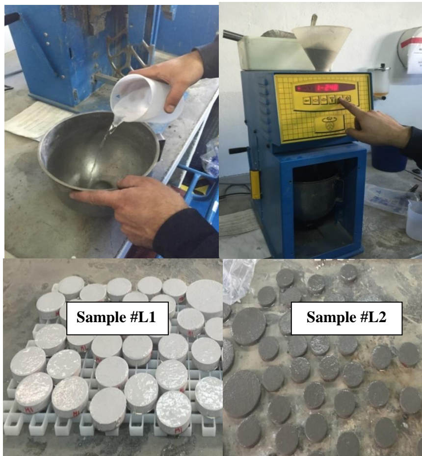
Figure 3. 4 Lab-made samples (#L1 and #L2) preparation following the procedure described on UNE-EN-196-1 and UNE-EN-197-1 standards.
