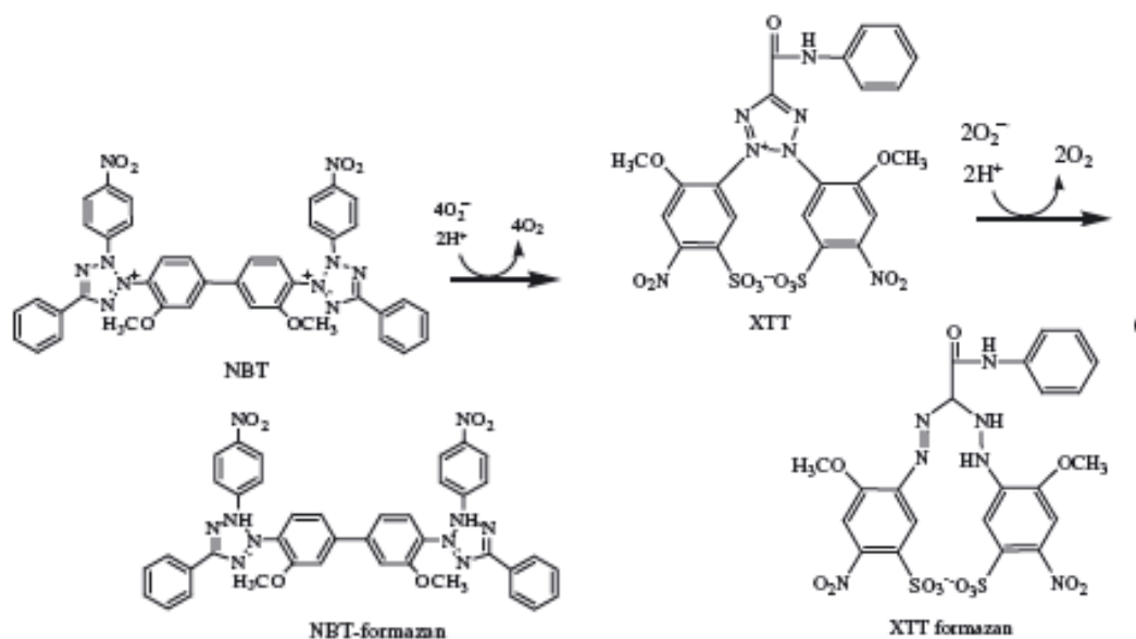
Figure 1. 22 Structure and reaction with superoxide radical of tetrazolium salts, Nitroblue tetrazolium (NBT) and 2,3-Bis(2-methoxy-4-nitro-5-sulfophenyl)-2H-tetrazolium-5-carboxanilide (XTT)[78].
