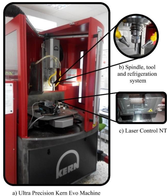
Figure 2.8 Ultra Precision Kern Evo Machine
