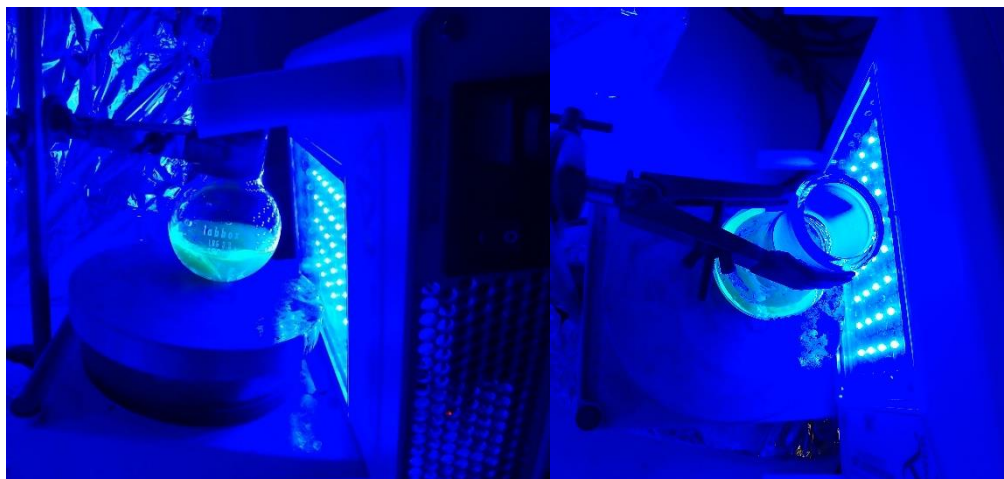
Figure 2.65. Reaction set-up with blue LEDs.
