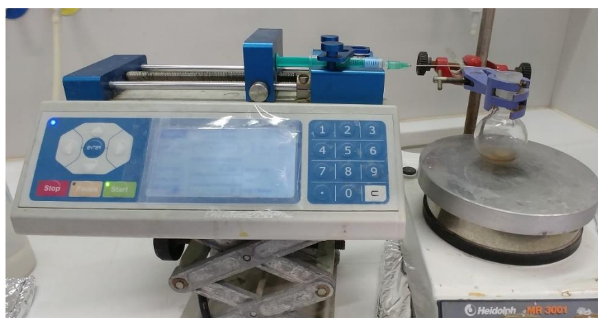
Figure 3.101. Addition of an aqueous solution of Oxone ® to the reaction mixture, using a syringe pump.
