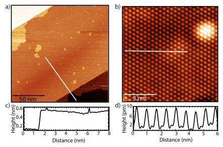
**Fig. 2 STM images of PdTe<sub>2</sub>. a** Large scale STM topographic image of the 1T-PdTe<sub>2</sub> surface ( $V_t = 1$ ,  $V_t = 50$  pA); **b** Atomically resolved STM image ( $V_t = 40$  mV,  $I_t = 1$  nA). Both STM images were taken at 1.25 K; **c** Line profile taken along the line in (**a**); **d** Topographic modulation along the line profile following the white line in (**b**).
