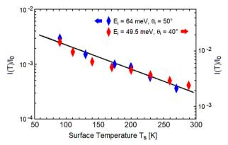
Fig. 4 E-ph coupling determination by the thermal attenuation of the He specular peak from PdTe<sub>2</sub>. Thermal attenuation of He-specular intensity of 1T-PdTe<sub>2</sub> measured along  $\overline{\Gamma}M$  at two different incident energies  $E_i$  and angles  $\theta_i$ . Note the shifted log scale for the two sets of data, so as to have a single average slope for all data and an average  $\lambda=0.58\pm0.05$ .
