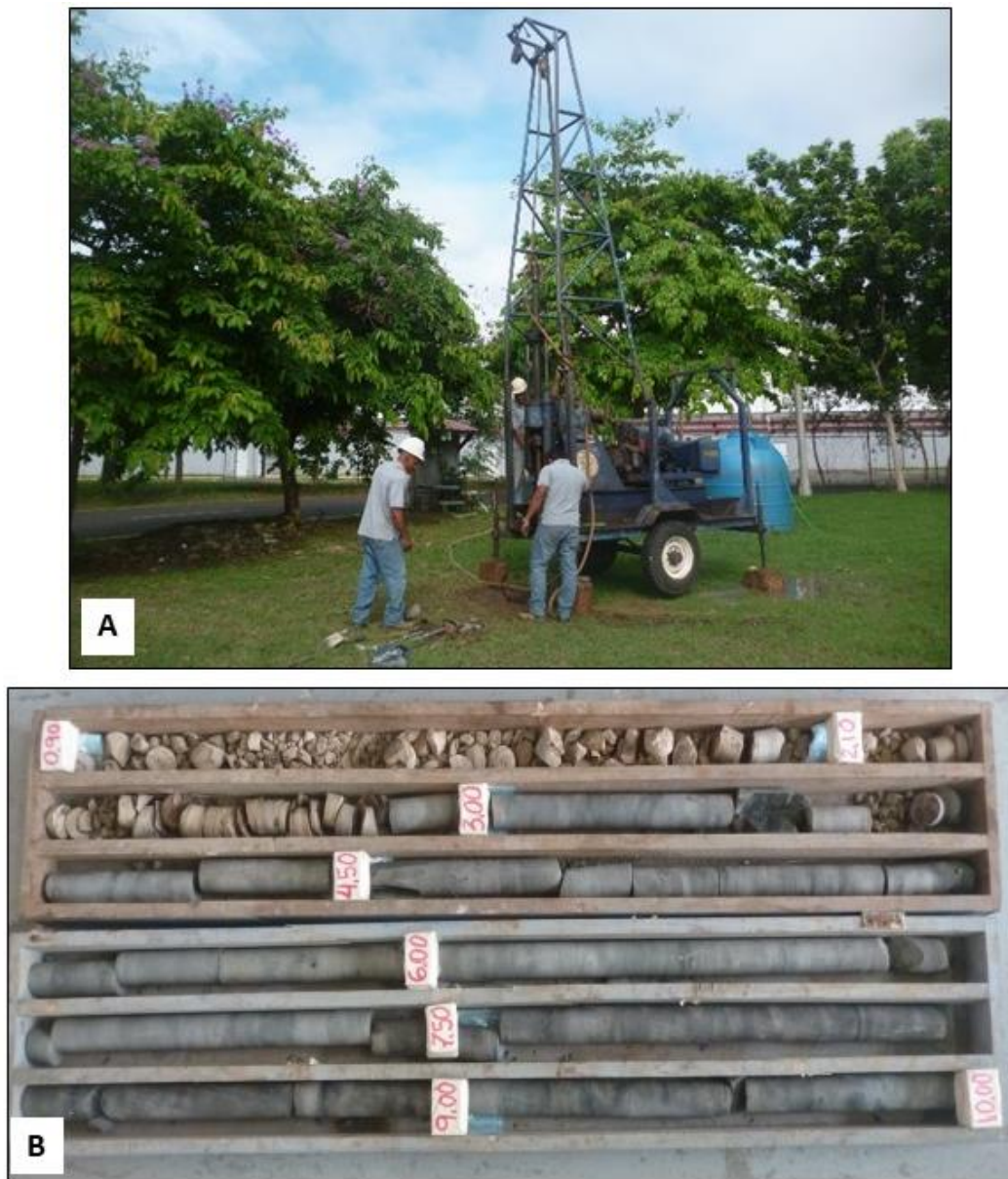
Fig. 4 Study area: a) Drilling of well; b) Drill hole profile.
