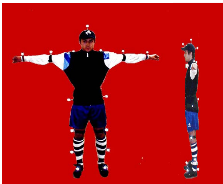
Figure 2. Location of the external markers to record motion with CLIMA optical tracking system
