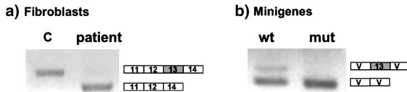
Fig. 1. Results of the RT-PCR analysis in fibroblasts (a) and in Hep3B cells transfected with wild-type (wt) and mutant (mut) minigenes (b). The schematic representation of the amplified bands is shown on the right of each gel. Numbers refer to the PCCA exons and V refers to exonic vector sequences.
