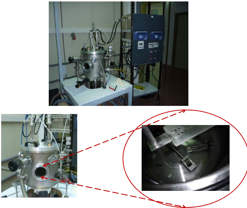
Figure # 2.4. Sputtering system with a zoom to the sample holder arm.
