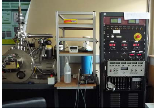
Figure # 2.2. Ion Beam Sputter Deposition system from Commonwealth Scientist Corporation at the INESC-MN facilities
