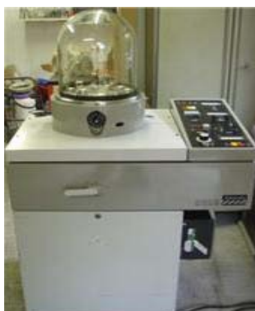
Figure 3.26. High vacuum coating system: Edward 306 evaporator.
