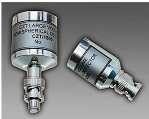
Figure 1.35. Photography of CdZnTe spectrometric detectors CZT/500 and CZT/1500.
