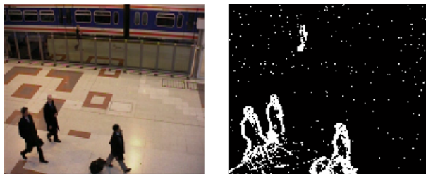
Figure 4.3: Obtained Foreground Mask with the modified basic background subtraction algorithm
