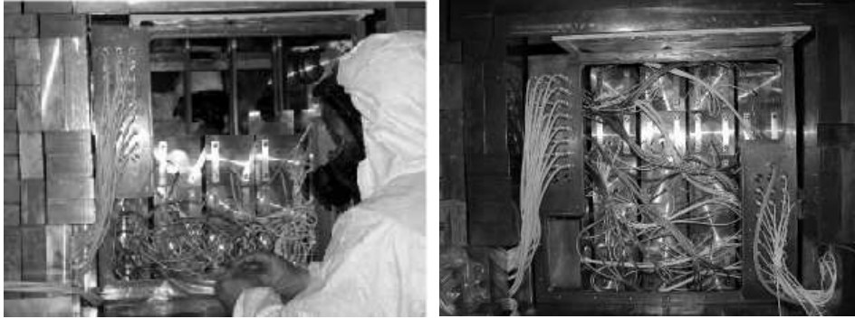
Figure 2.8: Left picture: during the LIBRA detectors installation in HP Nitrogen atmosphere. Right picture: view at end of the detectors installation. All the used materials have been deeply selected for radiopurity (see for example the cables with teflon envelop).
