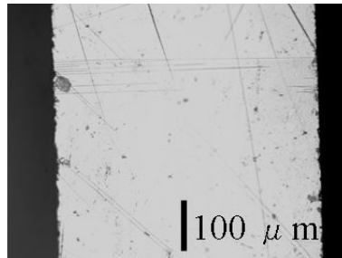
Figure 7.15: The polished edge (y-face) of the same sample as figure 7.14 is shown. Some domains can be seen along the depth of the substrate, but most of them are only seeds that do not reach the other face.
