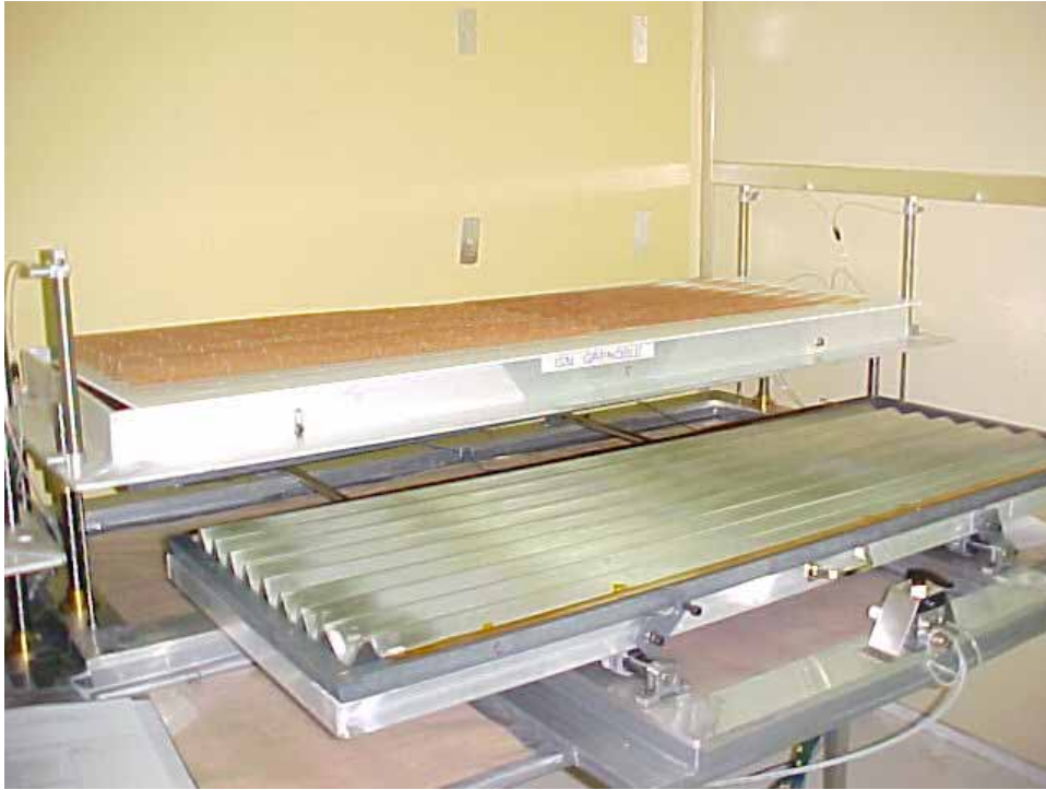
Figure 3.30: Picture of the high voltage test bench for outer wheel spacers.
