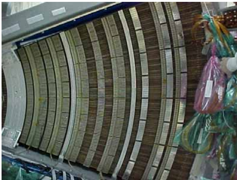
Figure 3.26: Front (back) side of a stacked module with all HV and SB cards plugged in, on the top (resp. bottom).
