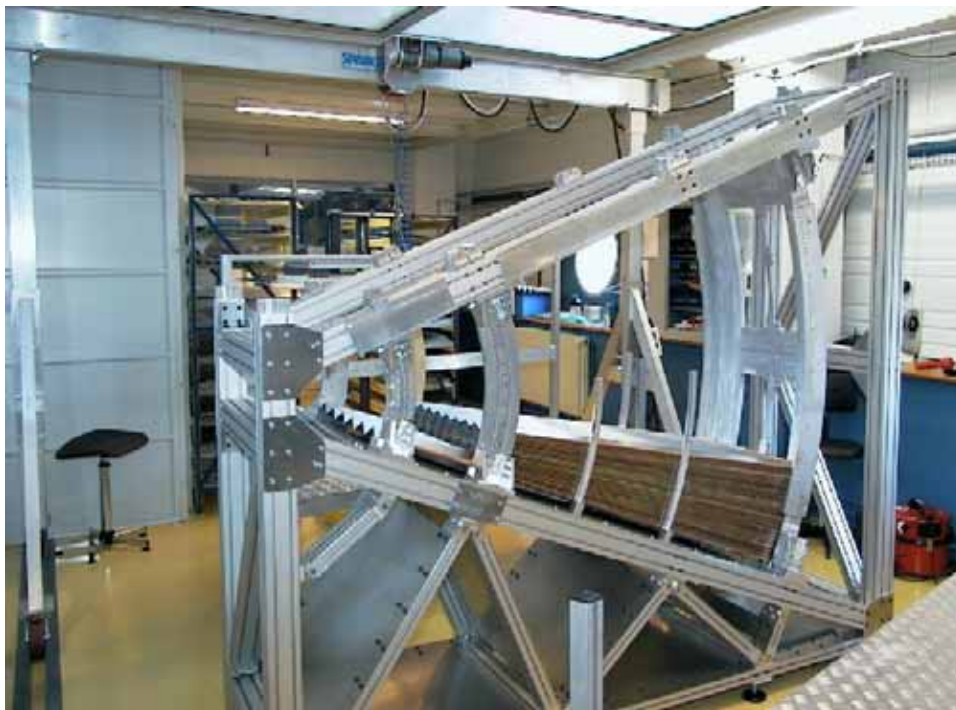
Figure 3.29: Structure elements bolted to the stacking frame (back side).
