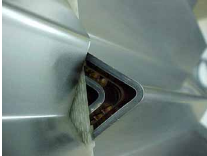
Figure 4.31: Photograph of an electrode sandwiched between two consecutive absorbers thanks to the spacers.
