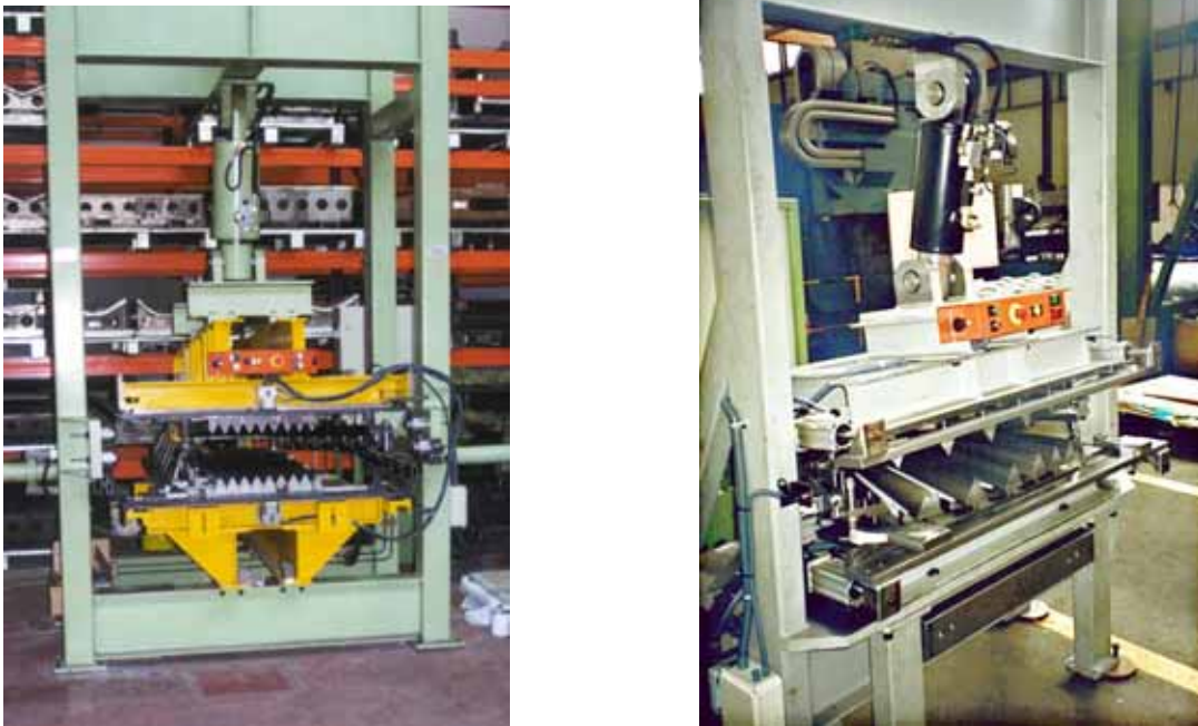
Figure 3.13: Presses used to bend large and small absorbers into accordion geometry.
