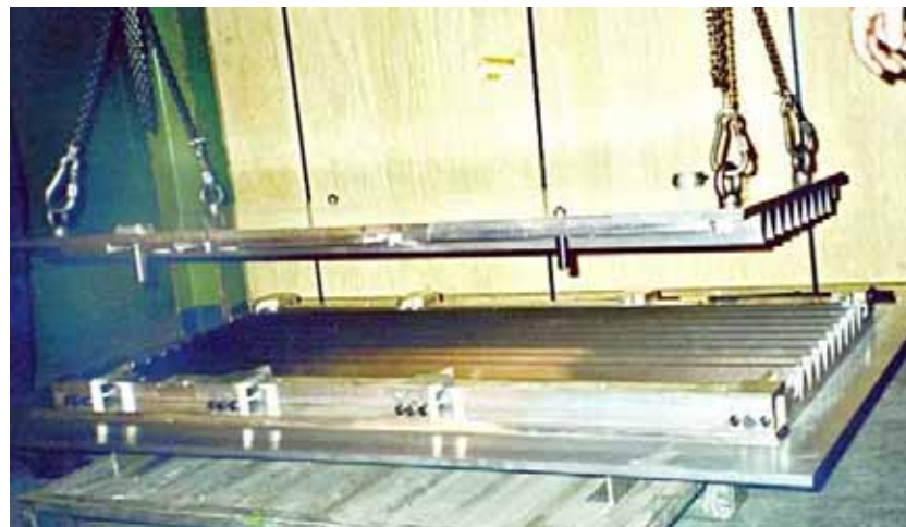
Figure 3.15: Mould with pre-glued absorber.
