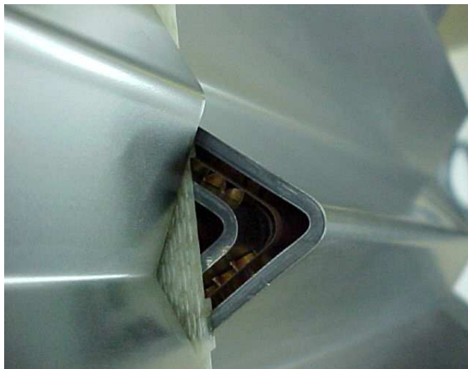
Figure 5.3: Stacked layer of the inner wheel. The electrode is placed in between two absorbers.
