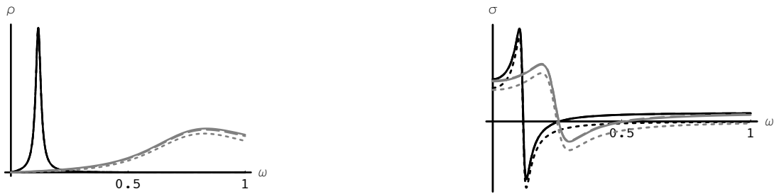
Figure 5.12: Imaginary (left) and real (right) parts of the retarded G_{tt,tt} correlator as a function of the frequency at q = 0.2 (black) and q = 0.4 (grey) for the real part and q = 1 (grey) for the imaginary part. The dotted line is the hydrodynamic mode contribution, the solid line is the exact solution and the dashed line is the four-mode approximation.
