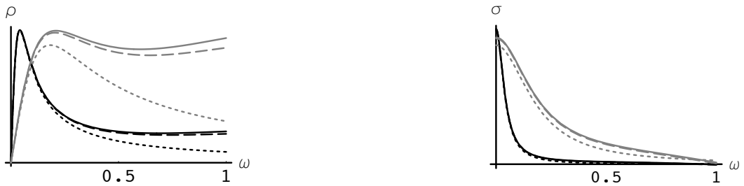
Figure 5.3: Imaginary (left) and real (right) parts of the retarded G_{tt} correlator as a function of the frequency at \mathfrak{q} = 0.2 (black) and \mathfrak{q} = 0.4 (grey). The dotted line is the hydrodynamic mode contribution, the solid line is the exact solution and the dashed line is the four-mode approximation.
