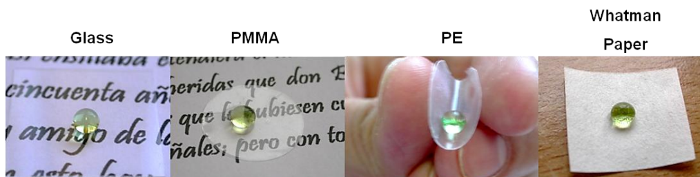
Figure VI-1: Images showing the appearance of superhydrophobic coatings prepared by spin-coating and spray-coating on glass, PMMA, PE, and Whatman paper.
