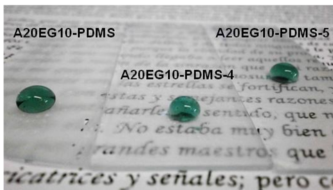
Figure V-9: Picture showing transparency and wettability of the coatings; A20EG10-PDMS, A20EG10-PDMS-4, and A20EG10-PDMS-5.
