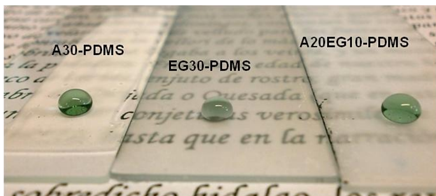
Figure V-10: Picture showing transparency and wettability of the coatings; A30-PDMS, EG30-PDMS, and A20EG10-PDMS.
