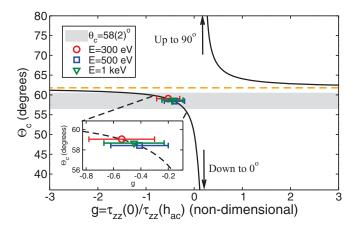
FIG. 6. (Color online) Dependence of the critical angle  $\Theta_c$  with the stress ratio g, Eq. (25). The horizontal gray bar indicates the experimental critical angle range for Xe<sup>+</sup>  $\rightarrow$  Si ( $\theta_c = 58 \pm 2^\circ$ ). The symbols show values from MD simulations, see legend. The inset is a zoom to show the weak dependence of  $\theta_c$  with E. The orange dashed horizontal line is a guide to the eye with asymptote  $\theta = 61.8^\circ$ .
