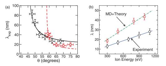
FIG. 8. (Color online) (a) Experimental ripple wavelength vs  $\theta$  for Si at 500 eV, using Ar<sup>+</sup> (black circles, from Ref. [11]) and Xe<sup>+</sup> (red squares) ions. The solid black and the dashed red lines are fits to Eq. (27) for  $\theta_c = 46^\circ$  and 58°, respectively. (b)  $\lambda$  vs *E* for Xe<sup>+</sup> according to Eq. (26) using MD data (red squares) and experiments (black circles). Straight lines are linear fits.
