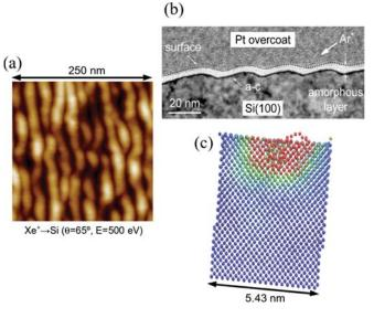
FIG. 2. (Color online) (a) AFM top view of experimental ripples obtained by Xe<sup>+</sup> IBS of Si for E = 500 eV and  $\theta = 65^{\circ}$ . (b) HRTEM cross-sectional high-resolution image along the  $\langle 110 \rangle$  direction. The free interface is marked by dots. (c) MD simulation after one Xe<sup>+</sup> impact under the same conditions as in (a). Different colors stand for different values of the temperature, which decreases with distance from the ion entry.
