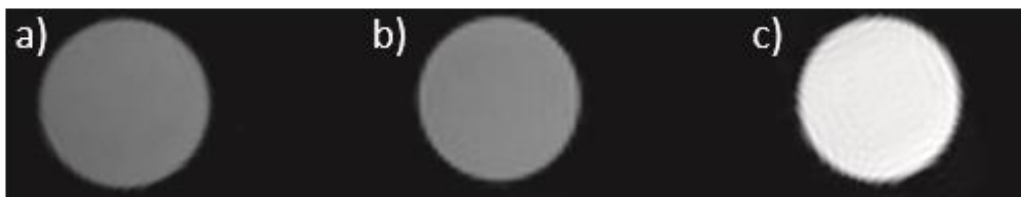
Figure 50. T_1 -weighted MR image of capsid buffer (a), compound 40 (b) and CCMV- 42 (c). Conditions: [Gd^{3+}] = 45 \mu M . Images at 600 MHz (14.1 T, TE = 6 ms, TR = 500 ms).
