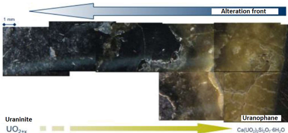
Figura 2-12. Image of the alteration front of an uraninite to an uranophane. Dark-Field Optical Microscopy (Quiñones et al. , 2003).
