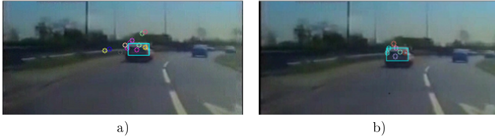
Figure 3.2: Points features: a) without spatial filtering and b) with spatial filtering.
