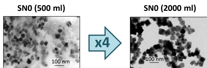
Figure 3.17. TEM micrographs for magnetite nanocrystals prepared in 500 ml and 2000 ml reactors.
