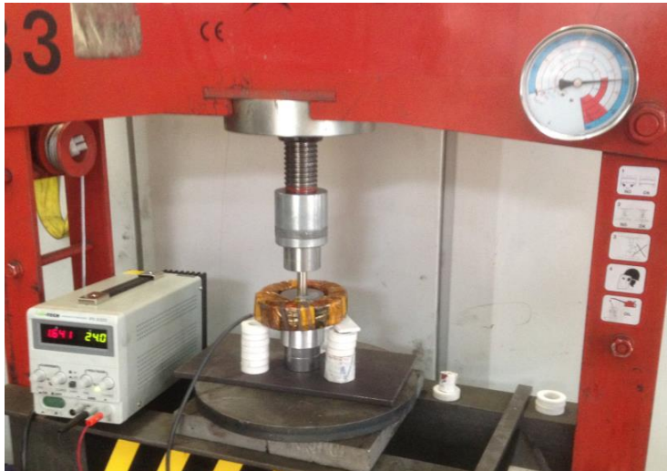
Figure 8.3: Hidraulic press applying pressure to the powder to form a magnet. At the same moment, a magnetic field is being applied to the powder under compaction too.
