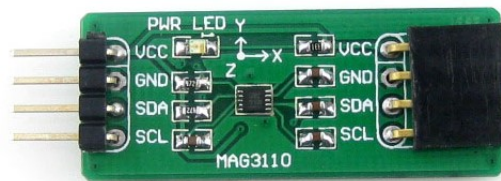
Figure 9.2: Image of a PCB containing the sensor MAG3110. This circuit is directly connected to the microcontroller using an I2C communication protocol.
