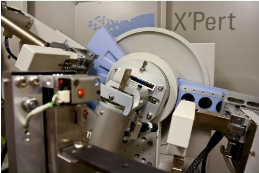
Figure 1.3: Picture of the device used on \theta - 2\theta XRD experiments. This image is courtesy of Sidi-UAM
