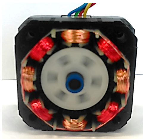
Figure 8.9: Image of the stepper motor while in operation. This stepper was modified with a home-made 3d-printed rotor containing 6 polymerized cobalt ferrite magnets.
