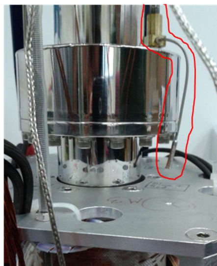
Figure 5.8. a) Image of the schematic view of the VTI. b) Image of the gas flow entrance (highlighted in red) that access directly to the helium bath.
