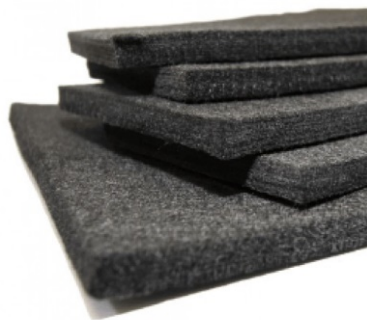
Figure 4.31 Carbon Felt material used as electrodes
