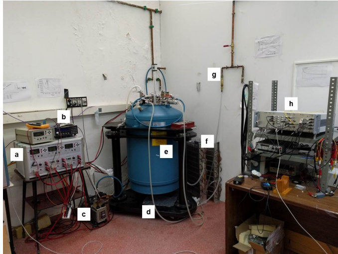
Figure 2.2: Picture of our set-up at the lab. In the image are shown the electronics to control the superconducting magnet (a), the temperature controller (b), the mechanical pump used to control the gas flow in the VTI (c), the isolation stage (d), the cryostat (e), the heaters to warm the cold He pumped from the VTI (f), the He recovery line (g) and the electronics of the LT-AFM (h).
