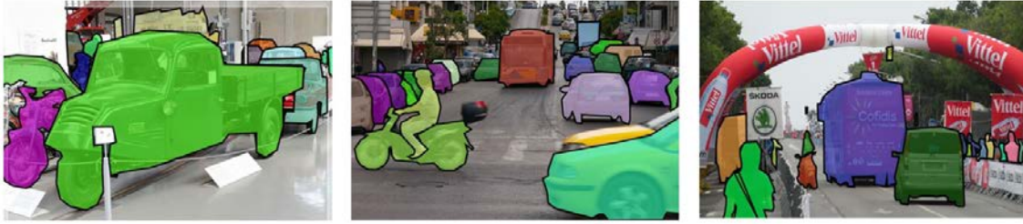
Figure 3.5: Example of the labeled image that contains the COCO dataset for car, motorcycle, truck and bus classes (for further references see www.cocodataset.org )
