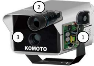
Figure 4.1: KOMOTO C7S with the different objects that make up this device (1: Jetson TX2, 2: Daheng Imaging Camera, 3: KOMOTO strobe).
