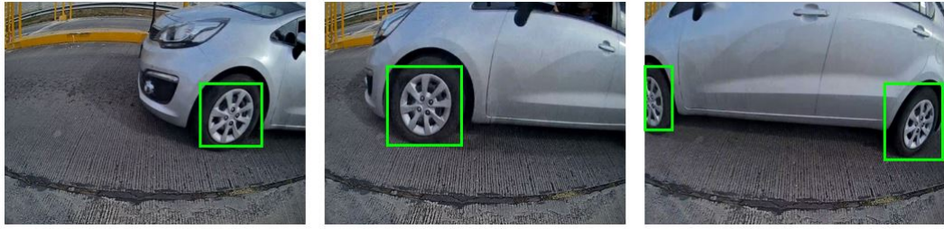
Figure 3.7: Example of frames of the video used to retrain the original CNN called "ssd mobilenet v1 coco" with the manual location of the axles.
