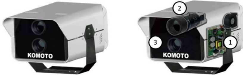
Figure 4.11: KOMOTO C7S. The left image represents the appearance and the right image represent the different objects that make up this device (1:Jetson TX2, 2:Daheng Imaging Camera, 3:KOMOTO strobe).
