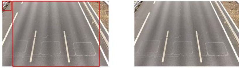
Figure 3.9: Example of filter detections by size with FGBG detection. The left image corresponds with bad detections obtained with FGBG because of a blur of the image in the capture process. Right image corresponds to the detection output after the filter by size process.
