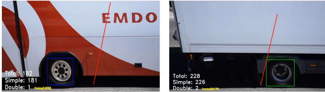
Figure 5.8: Example of the axle classification algorithm. The image on the left corresponds to a correct classification of a double axle and the image on the right corresponds to the error when classifying a double axle as simple.
