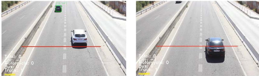
Figure 5.10: Example of two undetected vehicles with the back camera algorithm for the Scenario3 rear video.
