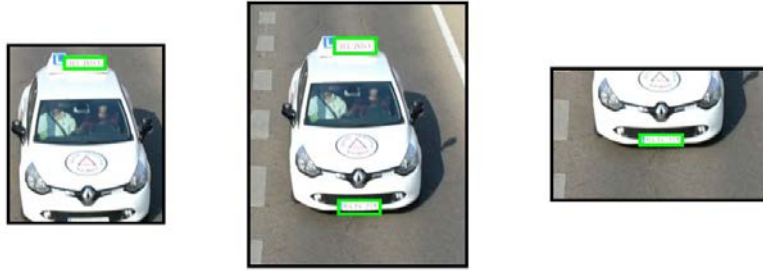
Figure 3.19: Example of image modification to calculate OCR. Starting from the left, in the first image, we have a plate miss detection, and, in the second one, we have a wrong detection in which it detects an another chain of characters as the plate.
