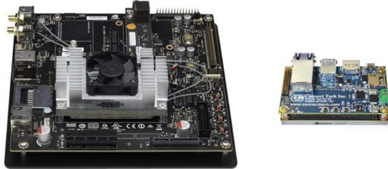
Figure 4.2: Both figures represents a device with a Jetson TX2 processor (the scale between them it is realistic). The device on the left corresponds to the developer kit, with all the possible benefits. The device on the right corresponds to a simpler board to integrate in the C7S KOMOTO device.
