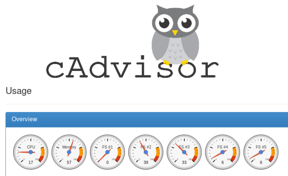
Figure 4. The cAdvisor interface management system provides users with an understanding of the use of resources and the performance features of their running containers. It is a running daemon that collects, accumulates, processes, and exports information about container execution.
