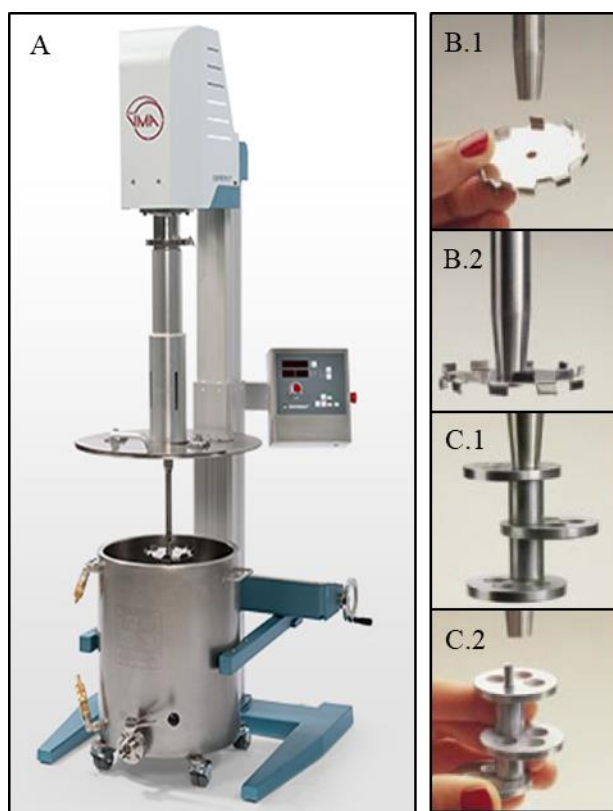
Figure 19. A. DISPERMAT ® CN 10 from VMA-GETZMANN GMBH. B. 1 and 2: Dissolver disc \varnothing = 40 mm. C. 1 and 2: Bead mill APS accessory.
