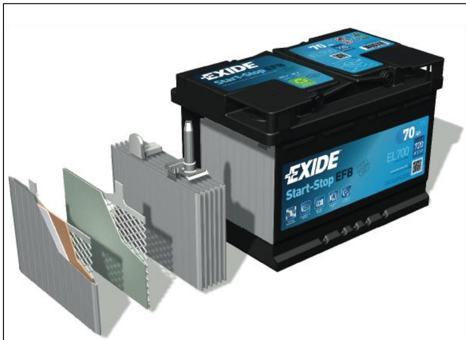
Figure 13. 12 V EXIDE Start-Stop EFB of 70 Ah. Flat positive plate covered by the pasting paper and surrounding by the separator. Flat negative plate covered by the pasting paper. Plate group [34].
