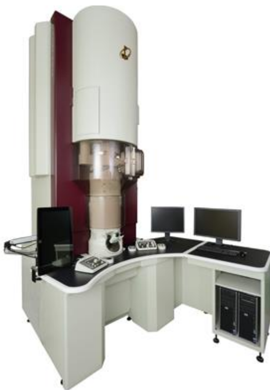
Figure 2.2. JEOL JEMARM200cF electron microscope.
