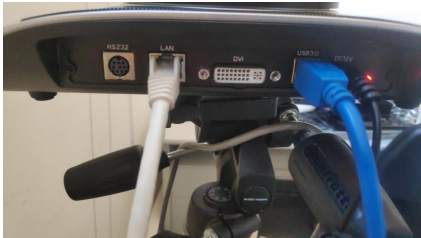
Figure 4-3: PTZ camera connections. The Ethernet cable comes from the switch. The USB3.0 is connected to the laptop.
