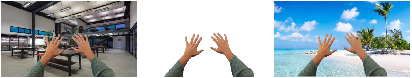
FIGURE 1. We propose semantic segmentation networks to segment human body parts (in this study the arms) to enhance self-perception in AV. Left: local reality; center: segmented arms; and right: AV with egocentric arms.
