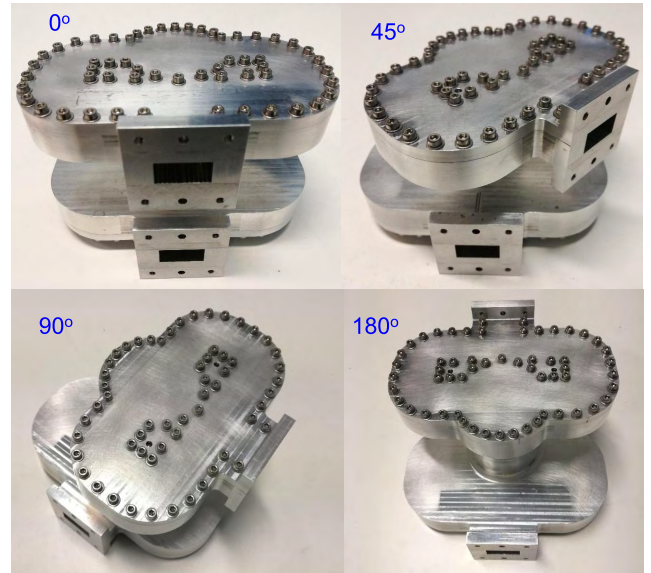
FIGURE 7. Back-to-back configuration of two similar transducers and four different angles between input and output ports ( 0^\circ , 45^\circ , 90^\circ and 180^\circ ) to verify the purity of the TM_{01} by means of the insertion loss and return loss measurements.
