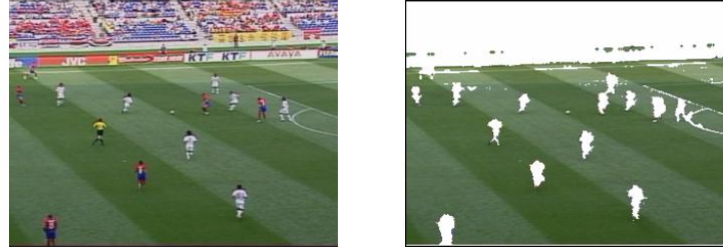
Fig. 2: Playfield detection result: Original frame (left) and the detected playfield pixels (right)
