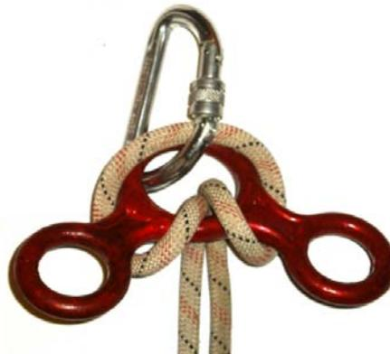
**Figure 12.** Double disengageable rappel.
