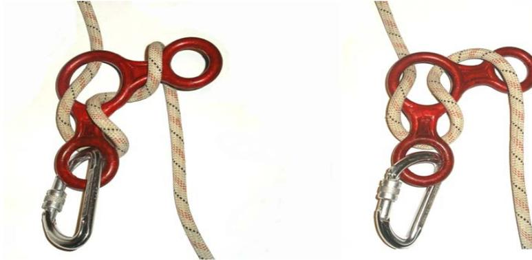
**Figure 11.** High friction (left) and middle friction (right) positions.
