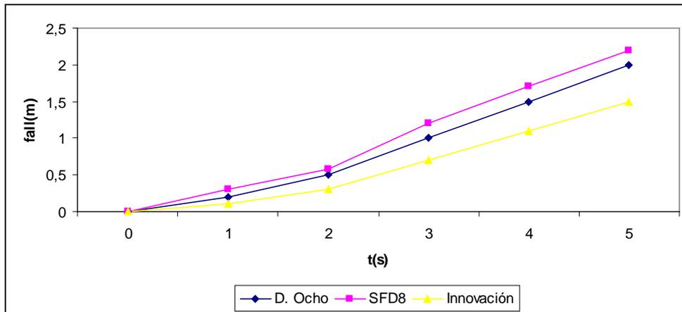
Figure 10. Difference of fall of a 80 kg weight in relation to the descender used.
