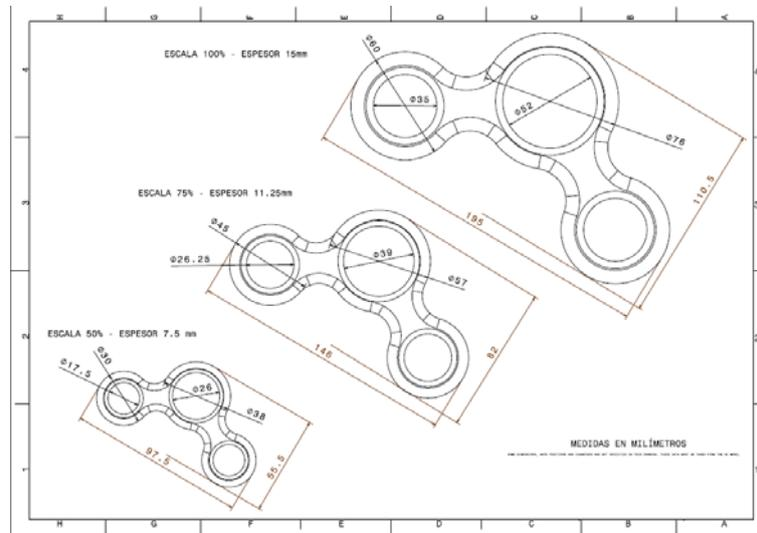
Figure 4. New descender layout in different scales.
