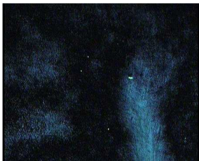
Figure 115. Texture of a 1:2 Pc-C 60 41 -Pc 37 blend between crossed polarizers at 140 °C cooling from the isotropic liquid.
