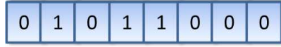
Figure 1: A Chromosome representing a community. Each allele represents a node of the graph and its belonging, or not, to the current community. In this example, a community built by three nodes of the graph is shown.
