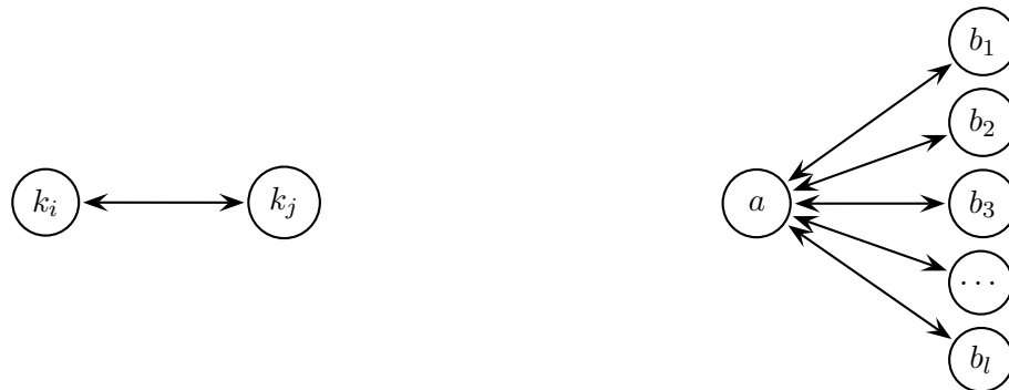
Figure 6.4: Pairwise classifiers (represented by bidirectional arrows) needed to calculate the pairwise class-posterior for context-independent classifiers (on the left) and context-dependent classifiers (on the right).
