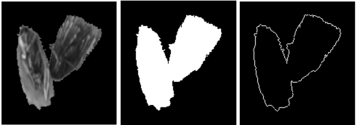
Figure 4.11: Contour extraction of two attached moths, the contour differs to contours of training examples which are single moth in each sample
