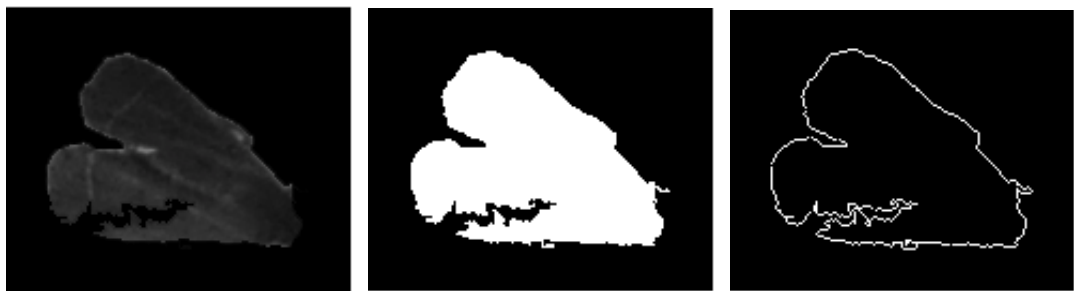
Figure 4.12: Contour extraction of an not complete moth caused by a background removing process
