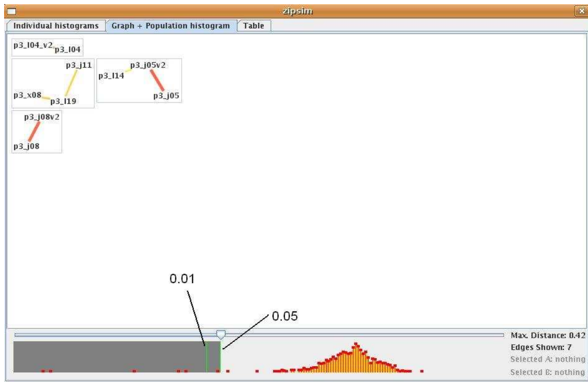
Figure 4.16: AC gives two threshold recommendations for plagiarism (outlier) detection in the Graph+Histogram visualization. The probability of a non-plagiarized pairwise distance falling below the threshold is annotated.
