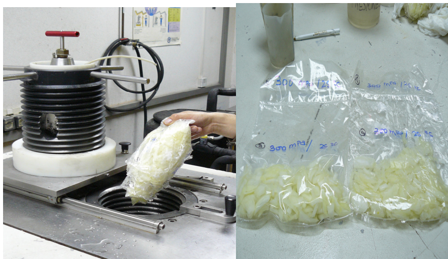
Figure 3. High-pressure processing (HP- Equipment at Instituto del Frío (CSIC) and samples packaged subjected to HP treatments)
