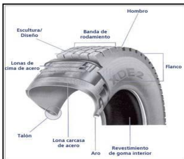
Figure 2.1. Parts of a tire.
