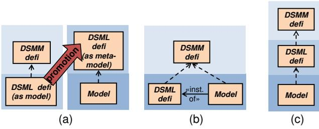
**Fig. 1** Some alternatives to define DSMM architectures. (a) Promotion transformations. (b) Merging the DSML meta-model and its instances in a single meta-level, to emulate the “instance of” relation. (c) Use of multi-level meta-modelling.
