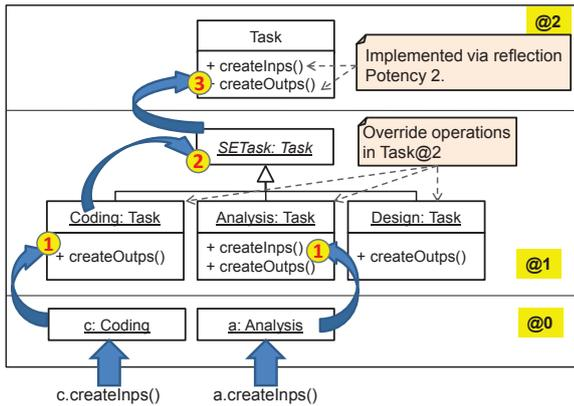
Fig. 18 Method overriding in a multi-level environment.
