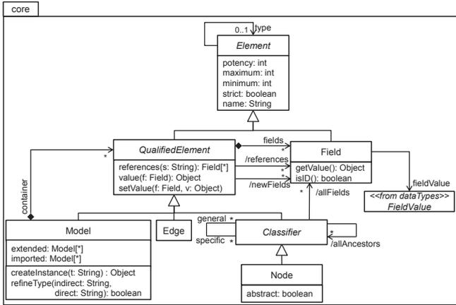
**Fig. 7** METADEPTH’s linguistic meta-model (simplified core package).
