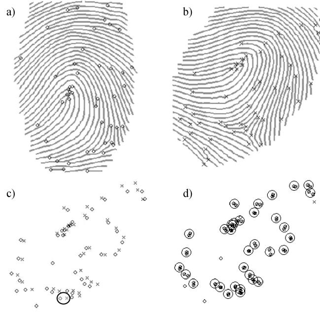
Figure 2.2: A generalized Hough transform based alignment. a) and b) shows the minutiae extracted from input and reference fingerprint; c) input and reference minutiae superimposed; d) circles denotes minutiae pairs mated using generalized Hough transform technique [Maltoni et al., 2009].
