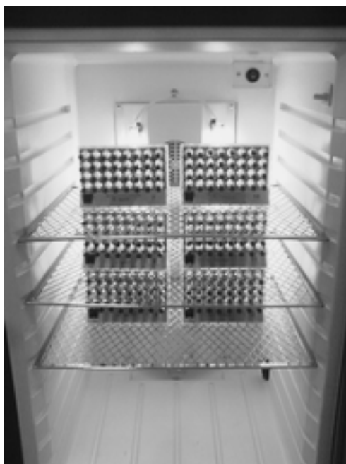
Figure 2.4: Experimental set-up of DAMS in incubator. A close up photo of six DAM2 monitors placed inside the incubator in preparation of an experiment (open door not shown), spread across three shelves. The incubator has a programmable daily lights on and off schedule to keep the circadian rhythm entrained; here seen with the lights on. Please note that these six DAM2 monitors have not been connected with cables to the PC yet.
