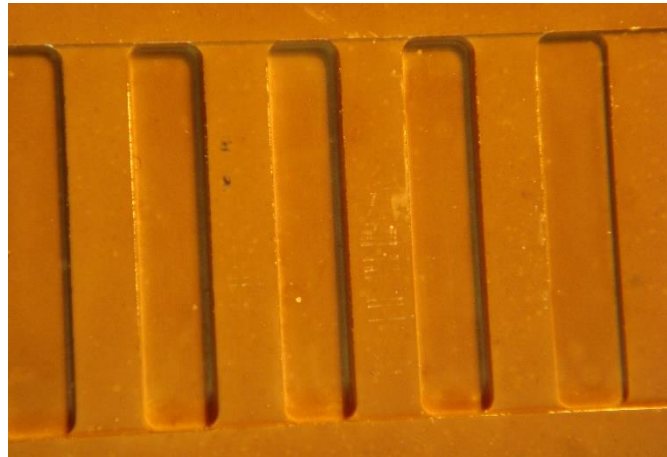
Figure 29. Detailed photo of MP4 with completed surface treatment in the central critical region
