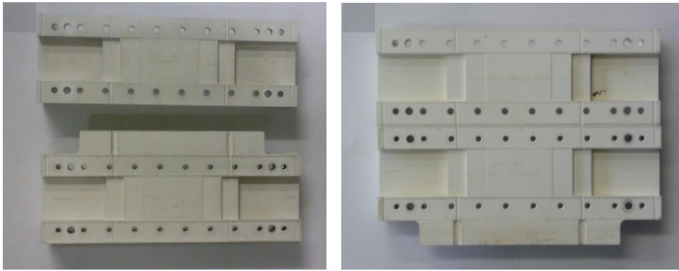
Figure 2. Photos of the first multipactor sample at various stages of chemical etching procedure. a) As received from Tesat, b) after chemical treatment, during second rinsing in deionised water, together with witness samples, c) after drying, before sending to ESTEC, and d) as received from ESTEC, where RF testing was performed.
