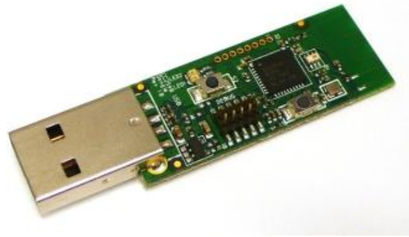
Figura 3.14: Módulo Bluetooth CC2540 (Texas Instrument).
