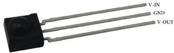
Figura 3.12: Receptor IR modelo TSOP4838 (Vishay Semiconductors).
