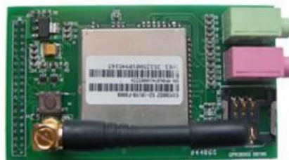
Figura 3.23: Módulo GPRS GPRS8000-S (Embest Technology).
