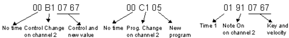
Figure 4: Example of three possible options for the second part of a track chunk [10]
