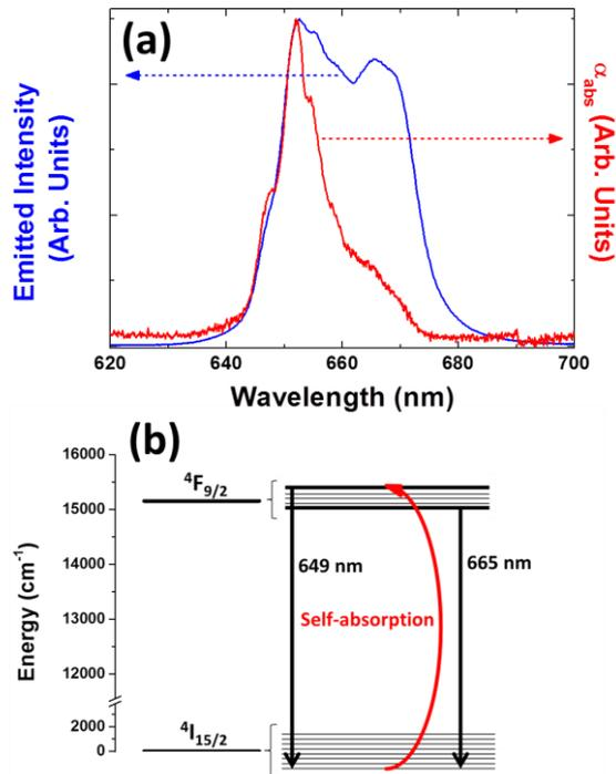
**Figure 6.** (a) Room temperature absorption and emission spectra of a colloidal suspension of UCNPs ( $10^{15}$  NP/cm<sup>3</sup>). (b) Energy level scheme of  $Er^{3+}$  ion in the  $SrF_2$  host. Just emission band corresponding to the  $4F_{9/2} \rightarrow 4I_{15/2}$  transition is shown. Both emission peaks are represented and those involved in self-absorption process are linked with a red arrow.
