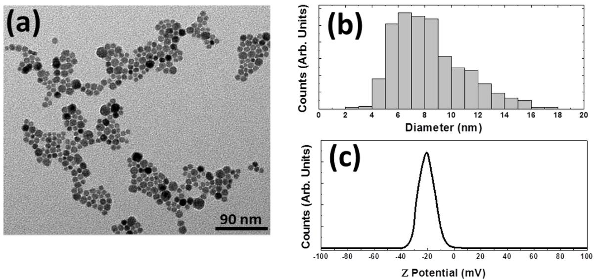
**Figure 1.** (a) TEM image of the UCNPs used all along this work. (b) Size histogram as obtained from the TEM images. (c) Z potential spectrum of the UCNPs used in this work.
