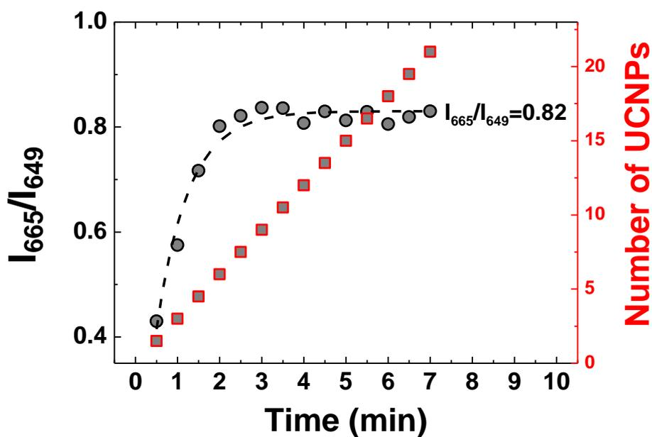
**Figure 5.** Ratio (gray dots) between the emitted intensities at 665 nm ( $I_{665}$ ) and at 649 nm ( $I_{649}$ ) as a function of the trapping time (data extracted from the emission spectra included in Figure 4b). Dashed black line is a guide for the eye. The evolution of the number of optically trapped UCNPs is included as red squares.
