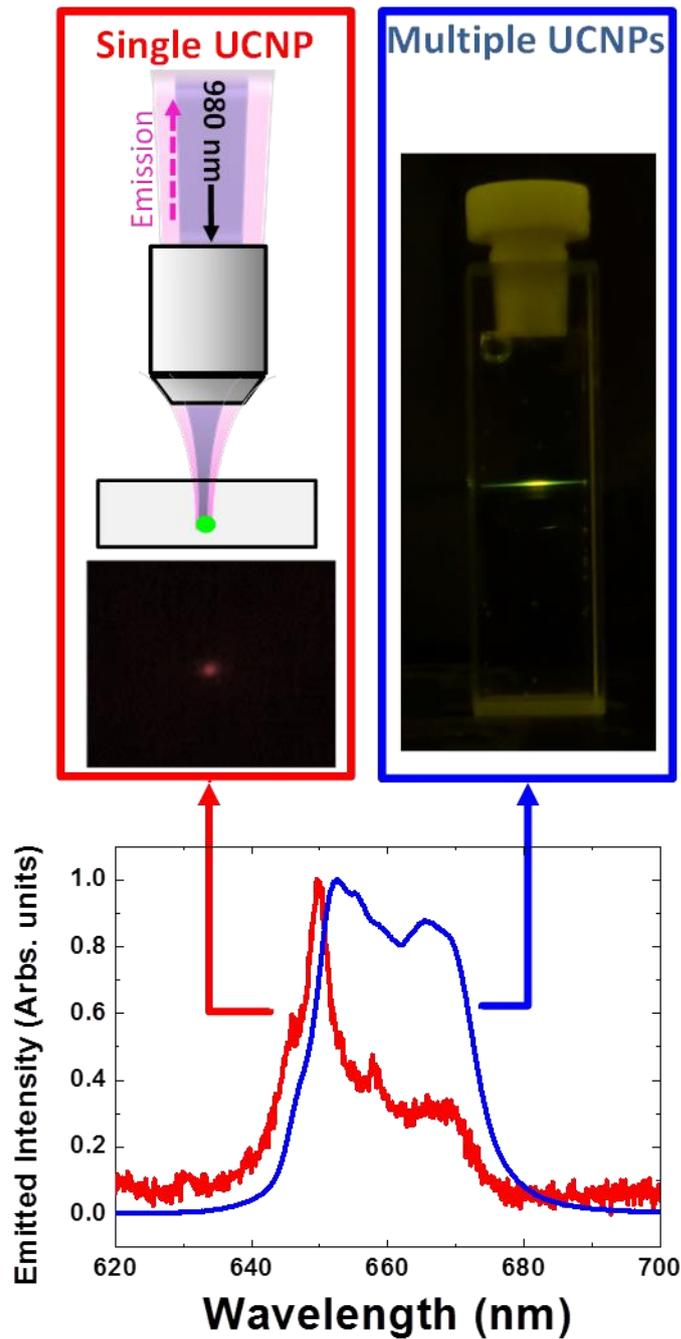
**Figure 3.** Upconversion emission spectra, as obtained from a single UCNP (red) and from multiple UCNPs (blue). Data were obtained from a single optically trapped UCNP and from a colloidal suspension of UCNPs ( $10^{15}$  NP/cm<sup>3</sup>), being the last one excited with a non-tightly focused laser beam. Excitation laser wavelength was, in both cases, 980 nm.
