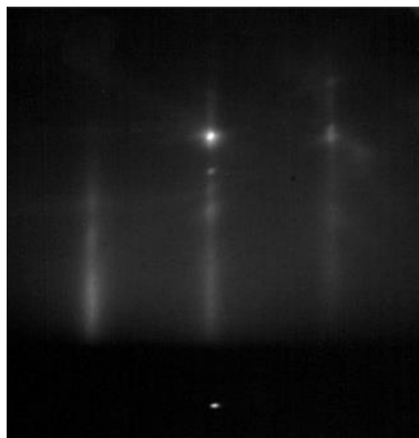
Figure 7.3. Characteristic RHEED diagram observed during the annealing of Si(111) at T_s = 650 °C.
