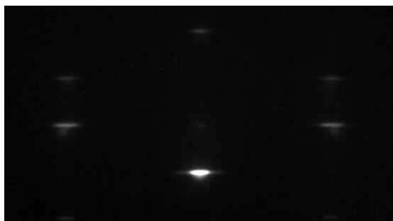
Figure 7.10. RHEED diffraction pattern observed during the growth of GaAs NWs.
